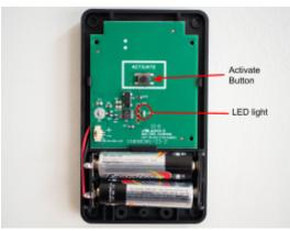
6. Front Cover Fitting: Ensure the front cover is positioned correctly (as per step 4) by starting at the top of the sensor case. There are two lugs on the top of the counter which clip into the cover to lock a secure fit. Then push the bottom part of the cover until it fits into place. With the mini screws provided, secure the cover to the base.
