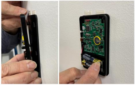
4. Now place the front cover back on. Ensure the front cover is positioned correctly by starting at the top of the sensor case. There are two lugs on the top of the counter which clip into the cover to lock a secure fit. Then push the bottom part of the cover until it fits into place. With the mini screws provided, secure the cover to the base as shown in the photo below.
