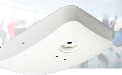
Our Overhead Thermal People Counters fit discreetly into the ceiling facing downwards and count the people that pass underneath using thermal technology. The sensors are designed to detect the heat emitted by people passing underneath it as infrared radiation.
