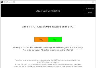
The IMMOTION Server is the IP address or DNS Name of the PC/Server where the IMMOTION software is installed. The default port for the IMMOTION Server is 55555.
