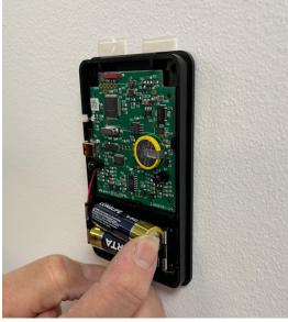
4. Now place the front cover back on. Ensure the front cover is positioned correctly by starting at the top of the sensor case. There are two lugs on the top of the counter which clip into the cover to lock a secure fit. Then push the bottom part of the cover until it fits into place. With the mini screws provided, secure the cover to the base as shown in the photo below.
