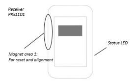
When the LED is blinking red you need to point the transmitter to the receiver until the LED lights up green continuously.
