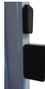
Flat/rear mount of Micro Counter (top) compared with side mount of PT Counter on door frame
