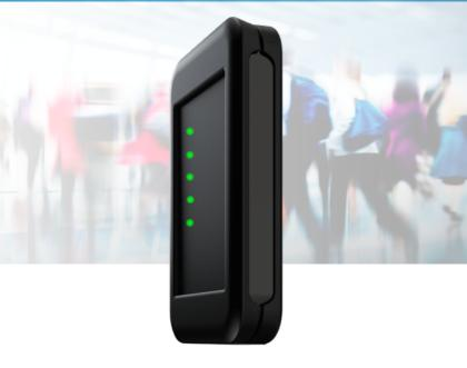
The Range Extender increases the Wireless Range between a Wireless People Counter (Network) and the SNG Hub (Sensor Network Gateway).
